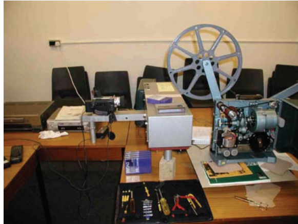
Figure 1. Heath Robinson-style digitisation: using a SONY Color Film Chain Adaptor, 16mm projector and a digital camera. Cambridge 2001.
